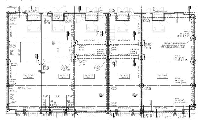
Figure 1 – South Side of Building Foundation Plan
