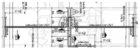
Figure 6 – Transfer Beams located on the Second Floor.
