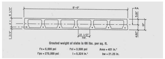
Figure 5 – Section Properties of Precast Planks
