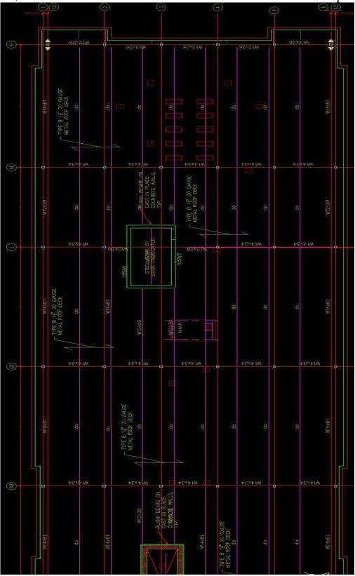
Figure 9B – South Side Structural Roof Framing Plan
