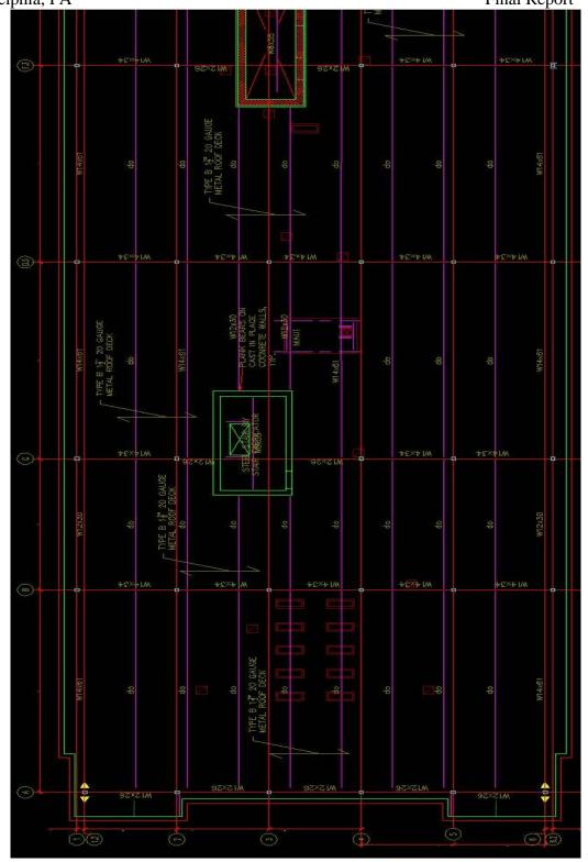
Figure 9A – North Side Roof Structural Framing Plan
